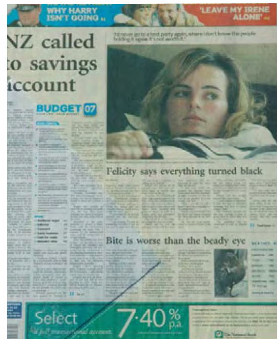
The above newspaper was left outside for two days. Standard glass was placed on top and then a small piece of our acrylic was placed on the glass across the bottom left corner. You can visibly see the UV fading to the newspaper through the glass.
